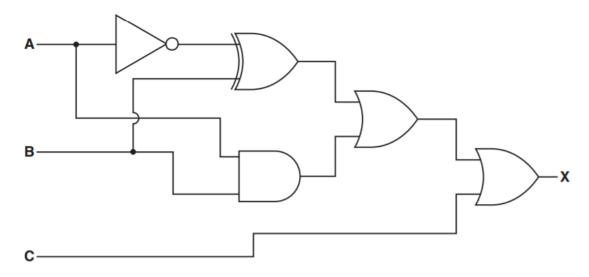
(a) Complete the truth table for the given logic circuit.
