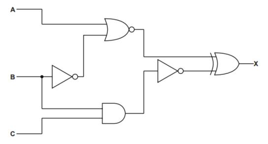
(a) Two NOT gates are used in the given logic circuit.
